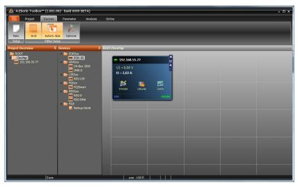
Figure 30: Device view enlarged with display of the menus PARAM, ONLINE and DATA
